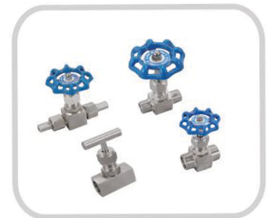
品名 (NAME) : 针型阀 NEEDLE VALVE 尺寸 (SIZE) : 1/8"-2" 材质 (MATERIAL) : CF8/CF8M 压力 (STANDARD) : 1000WOG/2000WOG/3000WOG 5000WOG/6000WOG 连接方式 (CONNECTION END) : M/M, F/M, F/F B/W, S/W
